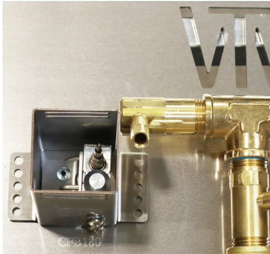
Photo 4a: Thermocouple Positioning
